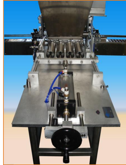
Piston Drive with Micro-Fill Adjustment
