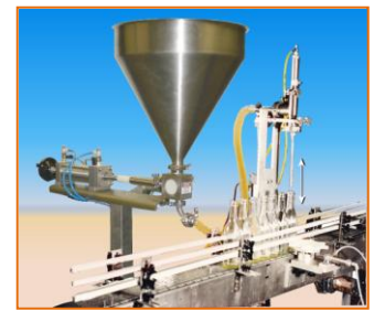
Diving nozzle mechanism
