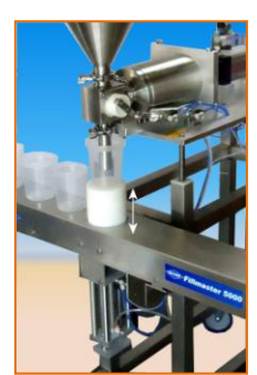
Container lift mechanism
