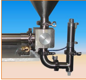
Positive cut-off filling nozzle
