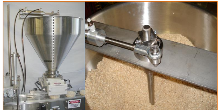
Agitator in hopper keeps product from bridging
